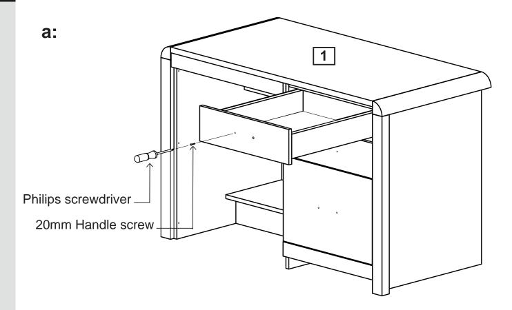
b: Replace the small bar handle on the front of the unit. Fix in position by screwing the 20mm handle screw into each small bar handle from inside the unit using a Philips screwdriver.
