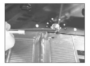
• Free the burners from their fixing screws.
