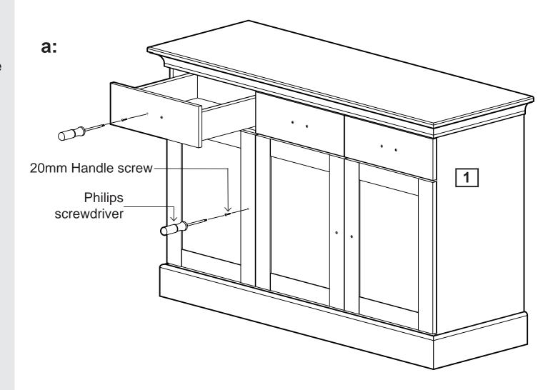
**b:** Replace the cup and oval handle on the front of the unit. Fix in position by screwing the 20mm handle screw into each cup and oval handle from inside the unit using a Philips screwdriver.
