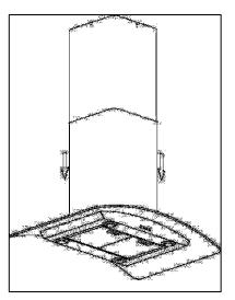
7) If you are going to be using the hood in extraction mode, you should fix the ducting hose to the spigot.
