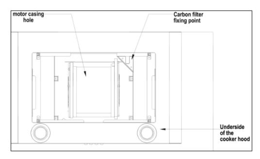
2) The line drawing above shows what you will see after removing the grease filters.
