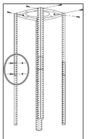
**3)** Extend the angle bars to the required height and then fix them in position using the 16 x M4 nuts and bolts with metal washers.
