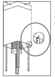
**4)** If your cooker hood is going to be used in extraction mode, then you should connect the ducting hose to the ceiling adaptor at this point.
