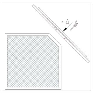
3) Use a screwdriver to take out the two screws that go through the fixing point and then lower the carbon filter over the motor casing hole.
