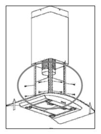
**6)** Lift the main body of the cooker hood onto the angle bar and then fix it into position using the 16 x M4 bolts.
