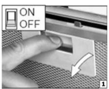
1) Remove the grease filters.
