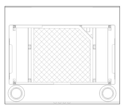
4) After fitting the carbon filter, the underneath of the cooker hood should appear as in the drawing opposite.
