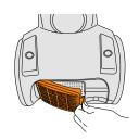
Push tab pull to remove the post-motor filter.
