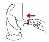
4 Take the Dispenser Cap of your choice (oval or star-shaped) and place it over the spindle with the vertical dial slightly slanted to the left (facing 11:00) and rotate clockwise into place. The dial should be vertically aligned with the chute (at 12:00) with the spout facing down.
