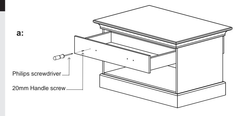
**b:** Replace the cup handle on the front of the unit. Fix in position by screwing the 20mm handle screw into each cup handle from inside the unit using a Philips screwdriver.
