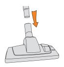
Insert the other end of the telescopic tube into the floor head.
