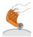
Tap the post-motor filter over a bin to release dirt/debris. Always replace before using your vacuum.
