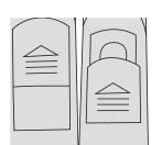
Slide vent cover on hose grip open to reduce suction if required.
