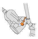
Place floor head into parking slot located at back of vacuum cleaner for storage and carrying.
