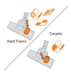
For use on carpets, click rocker switch forward. For use on hard floors click rocker switch back.
