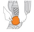
Remove the pre-motor filter. Separate the filter frame and foam.
