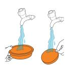
Rinse both the filter frame and foam under water (Max 40°C).
