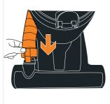
Attach the hose end to the floorhead ensuring it clicks into place. (All accessories can be used by either attaching them to the handle or the hose).
