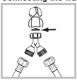
1. Connect the supply pipe to the water mains using a gas 3/4 attachment, fitting the rubber gasket and the filter supplied with the appliance and ensuring that they are fimly tightened to the taps. The water supply
