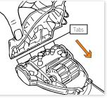
Detach lower housing and remove blockage.
