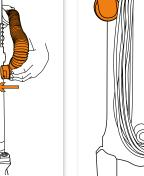
Connect the upper hose to the upper hose connector, rotate hose clockwise to secure.
