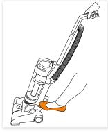
Place foot on the on/off button to switch the vacuum cleaner on.
