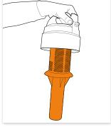
Turn the lid of the dirt container anticlockwise to remove.
