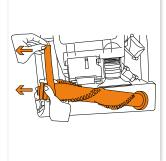
Lift the brush bar out of the base of the unit. Next, remove the belt from the brushbar and from the motor spindle towards the rear of the floor head. Replace the belt.
