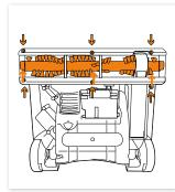
Turn unit over and remove the six screws using a crosshead screwdriver as indicated by arrows.
