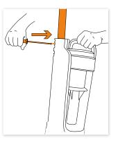
Using a crosshead screwdriver, remove the screw from the back of the unit as shown.
