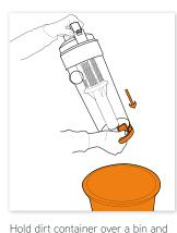
press the dirt container latch to open,
