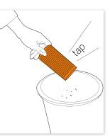
Tap the HEPA central filter against a bin to release dirt and then return to the unit.
