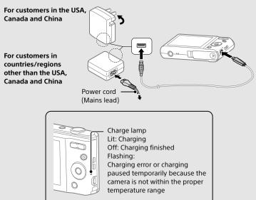
Connect the camera to the AC Adaptor (supplied), using the dedicated USB cable (supplied).
