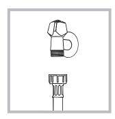
1. Connect the supply pipe by screwing it to a cold water tapusing a ¾ gas threaded connection (see figure).
