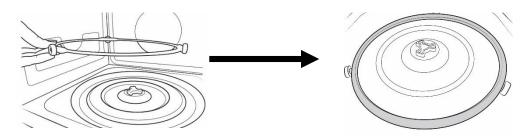
STEP 3) The glass tray should align with the turntable coupling
