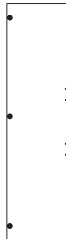
10 Mirror Door (D1030A) (1381 x 369mm) x 2 (Mirror - SG14 1376 x 311mm 4mm Safety Back SAR)
