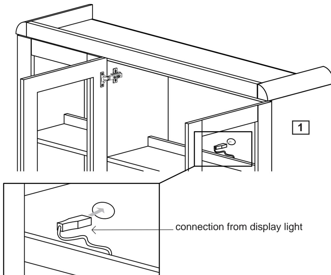
**b:** Connect the socket on the display light into the connection on the multi socket adapter **D**. You can now connect to the mains.
