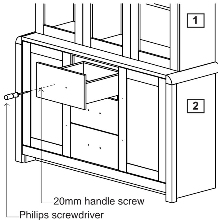
**b:** Replace the large and small bar handles on the front of the unit. Fix in position by screwing the 20mm handle screw into each handle from inside the unit using a Philips screwdriver.
