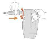
Small tools can be attached via concentration nozzle, twist clockwise until locked into position and secure. To remove concentration nozzle, turn anticlockwise
