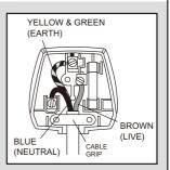
The wire which is Colored Yellow & Green must be connected to the terminal which is marked E or colored Yellow & Green. The wire which is colored blue must be connected to the terminal which is marked L or colored brown. Always ensure that the plug cord grip is fastened correctly. If a 13A (BS 1363) fused plug is used it must be fitted with a 13A fuse conforming to BS1362 and be ASTA approved. If in doubt contact a qualified electrician.
