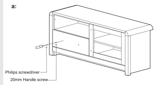
**b:** Replace the large bar handle on the front of the unit. Fix in position by screwing the 20mm handle screw into each large bar handle from inside the unit using a Philips screwdriver.
