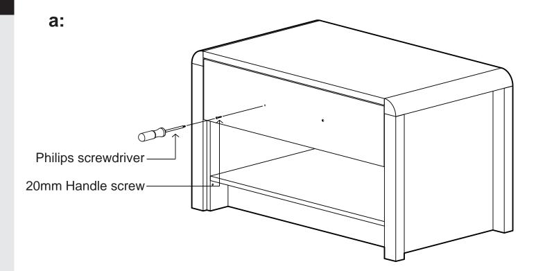
**b:** Replace the large bar handles on the front of the unit. Fix in position by screwing the 20mm handle screw into each handle from inside the unit using a Philips screwdriver.
