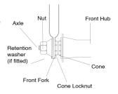
ensuring that the wheel is central within the forks. Refer to page 19 for recommended torque settings.
