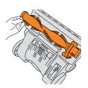
Lift the brush from the machine starting at the side without the belt on.
