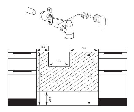
Connection to the cooker should be made with an approved appliance flexible connection to BS 669. A length of 0.9 to 1.25m is recommended. The length of hose chosen should be such that when the cooker is in situ, the hose does not touch the floor.
