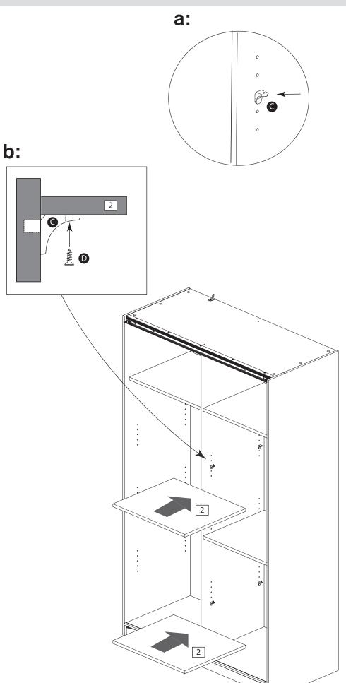
**b:** Position shelves 2 onto shelf supports **C** and fix by screwing eight chipboardscrews **D** through shelf supports **C** into shelves 2.
