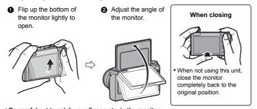
· Be careful not to catch your finger, etc. in the monitor. . When rotating the monitor, be careful not to apply too much force or drop the camera. This may cause scratches and malfunctions.
