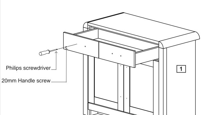
**b:** Replace the large and small bar handle on the front of the unit. Fix in position by screwing the 20mm handle screw into each bar handle from inside the unit using a Philips screwdriver.
