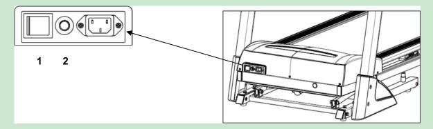
Plug in the mains power and turn on the switch (1). You will hear a signal tone and the screen of the Computer will light up.
