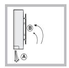
**AIR** maximises air circulation, improving the efficiency of the evaporator and helping to achieve the optimal temperature inside the refrigerator as quickly as possible each time it has been opened. The blown air (A) is cooled when it comes into contact with the cold wall, whereas the hotter air (B) is sucked up (see diagram).
