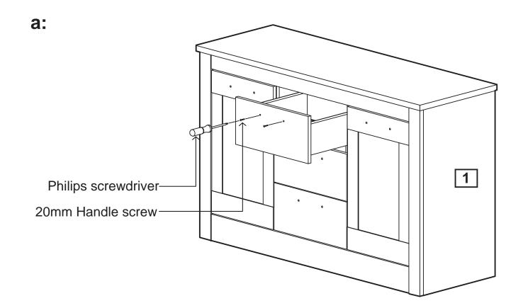
**b:** Replace the strap handle on the front of the unit. Fix in position by screwing the 20mm handle screw into the strap handle from inside the unit using a Philips screwdriver.
