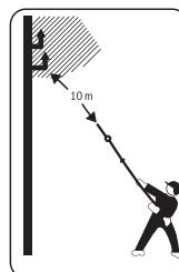
**Never touch power supply or telephone lines.** These lines conduct high voltage and there is severe danger of electric shock. Keep a minimum distance of 10 m.
