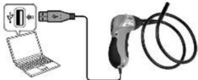
Connect inspection camera to USB port when requested.
