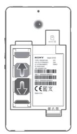
• Remove the battery cover and the battery, then insert the SIM cards into the corresponding slots with the gold-coloured contacts facing down.
