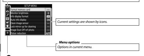
A description of the currently selected option or menu can be displayed by pressing the  $\mathbb{Q}^{\mathbf{x}}$  (?) button. Press  $\blacktriangle$  or  $\blacktriangledown$  to scroll through the display. Press  $\mathbb{Q}^{\mathbf{x}}$  (?) again to return to the menus.
