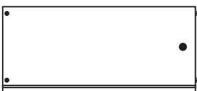
11 Large Right Drawer Side (W370-165RH) (370 x 165mm)
