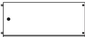
10 Large Left Drawer Side (W370-165LH) (370 x 165mm)
