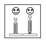
Screw the bolts D into the holes indicated on the sides 1 and 4 and the divider 2 and 3
