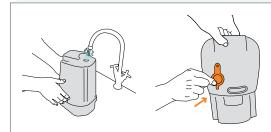
To clean dirty water tank ducting, place dirty water tank under a tap and dispense high pressure clean water into the completely, replace guick inlet port of the dirty water tank to loosen debris that has accumulated
