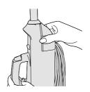
Insert the detergent tank back into the machine until it clicks into place.
