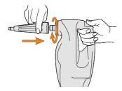
Small tools can be attached via concentration nozzle, twist clockwise until locked into position and secure. To remove concentration nozzle, turn anticlockwise.
