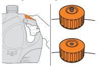
After using the steamer, press the power button to switch OFF and unplug the power cord from the mains. Release excess pressure by depressing the trigger before opening the water cap. The pressure indicator within the water tank cap will indicate all the pressure is released
