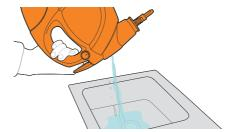
After allowing the steamer to cool for a minimum of 10 minutes, slowly start to unscrew the water tank cap anti-clockwise whilst gently pushing the trigger. DON'T FULLY UNSCREW THE WATER TANK CAP. When fully cooled and the pressure has been released, the water tank cap should turn freely to remove. Empty any residual water and allow the water tank to dry. Clean the external surface with a dry cloth
