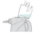
Slowly pour water into water tank. Do not overfill the water tank. Allow space to be left at the top
