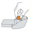
NOTE: For best results, fill with 200ml of detergent. Alternatively dilute the mixture with 80ml detergent and 120ml water
