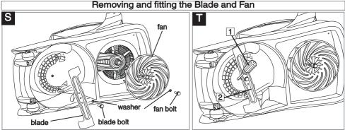
Switch off, wait until the blade has stopped rotating and disconnect from the mains electricity supply BEFORE attempting to remove or refit the blade.
