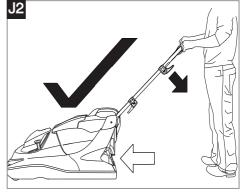
Push the spring assisted handles down for a better hover performance as illustrated in Fig J2
