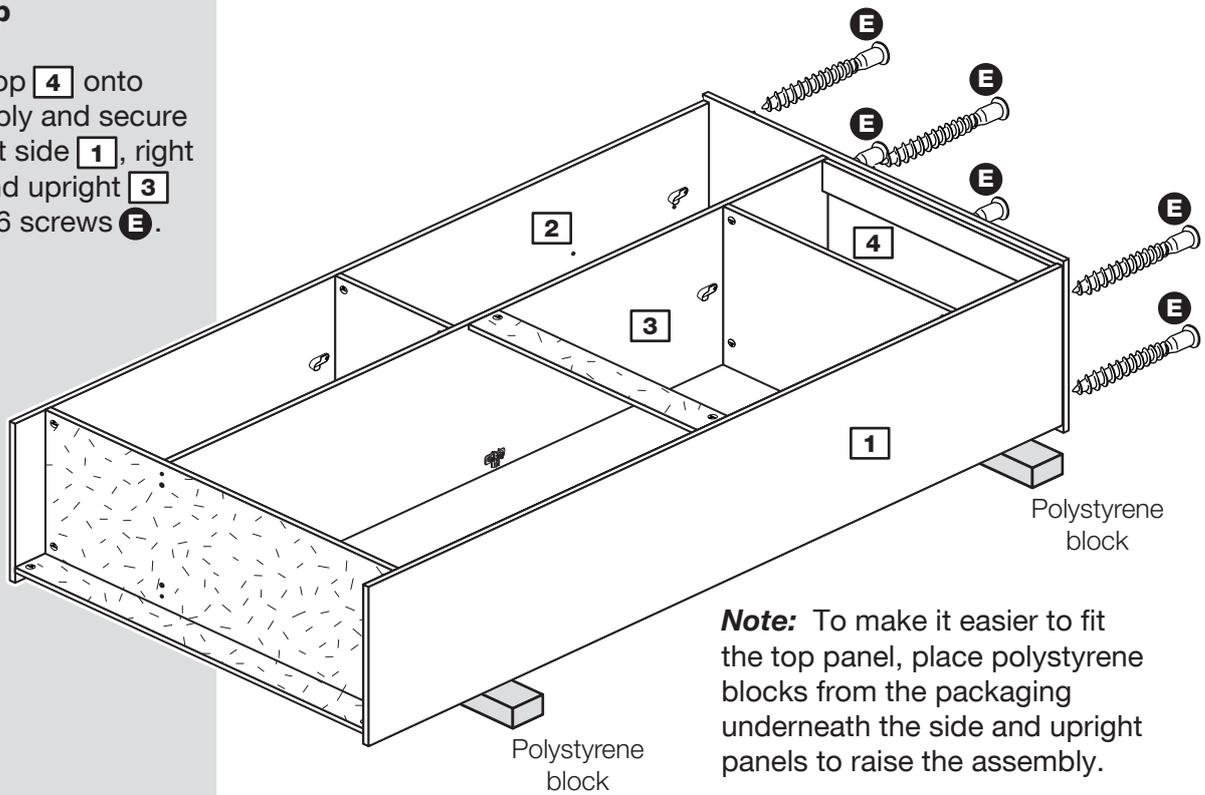
**Note:** To make it easier to fit the top panel, place polystyrene blocks from the packaging underneath the side and upright panels to raise the assembly.
