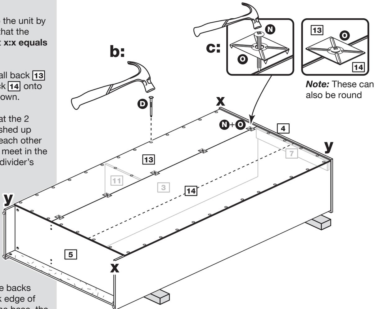
**b:** Nail **D** the backs onto the back edge of the 2 sides, the base, the small horizontal and the rail at the top.
