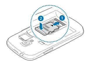
**3** Push the memory card down into the slot and then slide it backwards until it locks into place.
