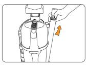
Remove extension tube from holder. Attach extension tube to hose.
