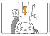
Push the lower back panel onto the base of the unit.
