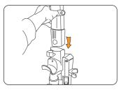
Attach handle to the back panel by pushing down firmly.
