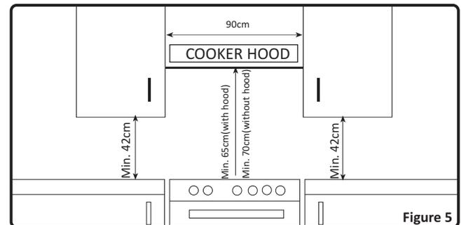
The cooking appliances that operate with gas, throw the burned gas wastes out directly to the outside or through the cooker hoods that are connected to a chimney that opens directly to the outside. If it seems not possible to install a cooker hood, it is required to set an electric fan on the window or wall that has access to fresh air. This electric fan must have the capacity to change the air of the kitchen environment 4-5 times of its own volume of air per hour.
