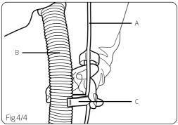
Push end of solution tube onto connective valve on the wash tool (Fig.4/5).
