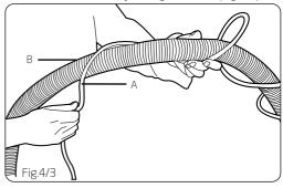
After wrapping the tube around the hose, affix solution tube (A) to hose (B) using clips provided (C) to hold it in place (Fig.4/4).
