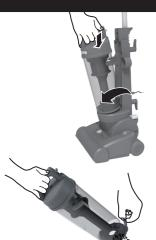
To remove the dust container from the cleaner, press the bin release button.
