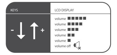
The new volume level is shown on the display for 2s then saved.
