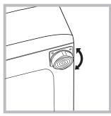
2. If the floor is not perfectly level, compensate for any unevenness by tightening or loosening the adjustable front feet (see figure); the angle of inclination, measured in relation to the worktop, must
