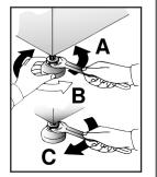
Note: we recommend you keep the screws to immobilise the machine for future transit. The Manufacturers will not be responsible for any possible damage to the machine caused by not following the rules relating to releasing the mechanism. The user is responsible for all costs of installation.
