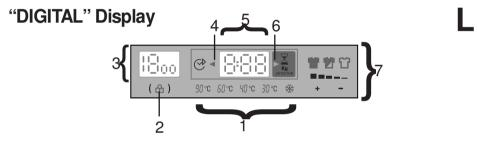
The display's indicator system allows you to be constantly informed about the status of the machine:
