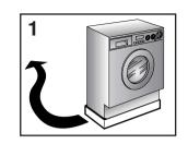
Remove the polystyrene base and place the machine near its permanent position (diagram 1).
