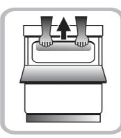
Before moving your cooker, switch off at the cooker control unit, ensure that it is cool. Open the grill door
