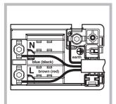
1 Open the terminal board by inserting a screwdriver into the bottom tabs of the cover. Use the screwdriver as a lever by pushing it down to open the cover (see diagram).
