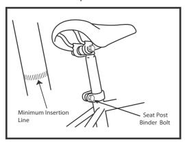
Loosen nut on the seat post binder bolt and add 3 or 4 drops of oil onto the threads of the bolt. Thread the nut on the seat post binder bolt loosely. Insert the seat post into the seat tube of the bicycle frame observing the minimum insertion mark on the seat post.
