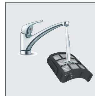
**STEP 6:** Leave the filter to dry for 24Hrs before re-fitting.
