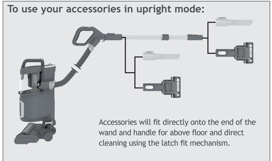
**IMPORTANT:** When using cleaning tools in upright accessory mode, please hold or support the cleaner in a safe position whilst using the wand.
