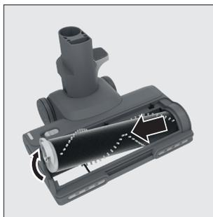
STEP 4: Remove the brushbar from nozzle and remove any excess debris.
