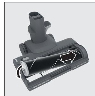
STEP 6: Refit the nozzle window. Locate the front edge first then 'click' into position at the back to ensure location.
