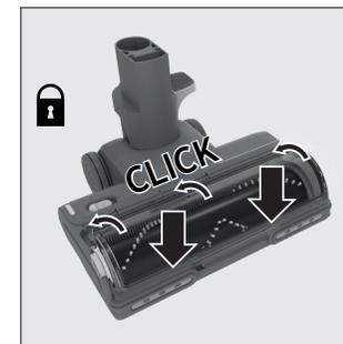
**IMPORTANT: IF THE NOZZLE WINDOW IS NOT RE-ASSEMBLED CORRECTLY, THE BRUSHBAR STATUS LIGHT WILL FLASH RED WHEN THE PRODUCT IS SWITCHED ON.**
